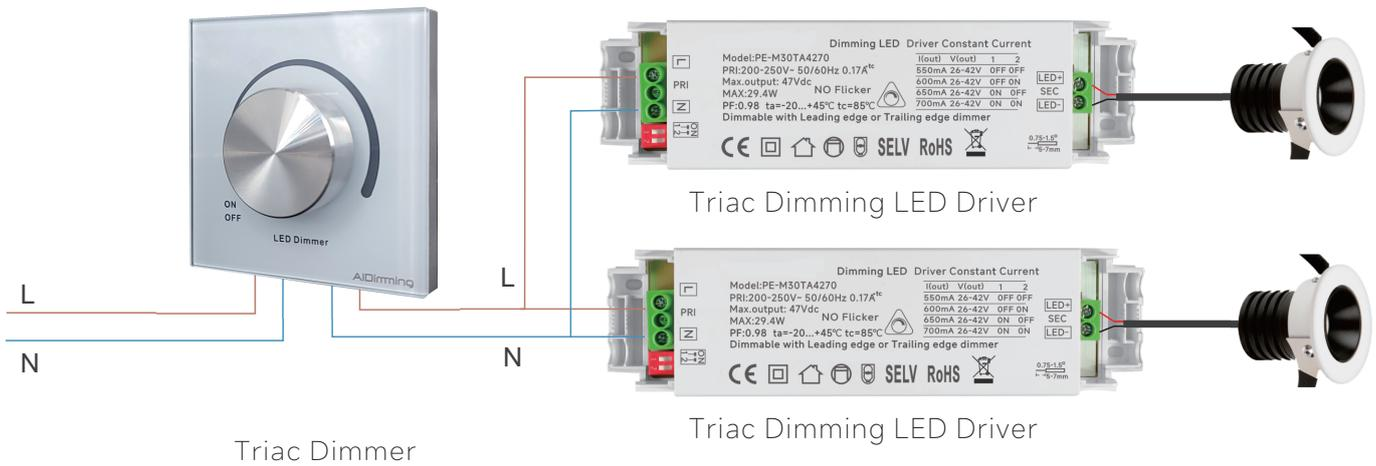
Note: there are two kinds of Aldimming brand dimmers, one is L, N in, L, N out (with infrared remote control), the other is L in, L1 out, thyristor dimmer;
