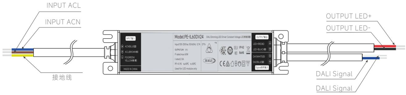
Note: the signal line interface cannot be connected to high voltage, otherwise the power supply will be damaged
